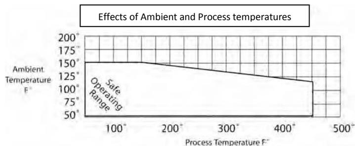
Figure 4: Ambient and Process Temperature Effect on Safe Operating Range
