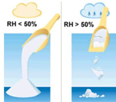
Figure 1: High Relative Humidity Combined with Hygroscopic Materials Make for Flow Problems in Vessels
