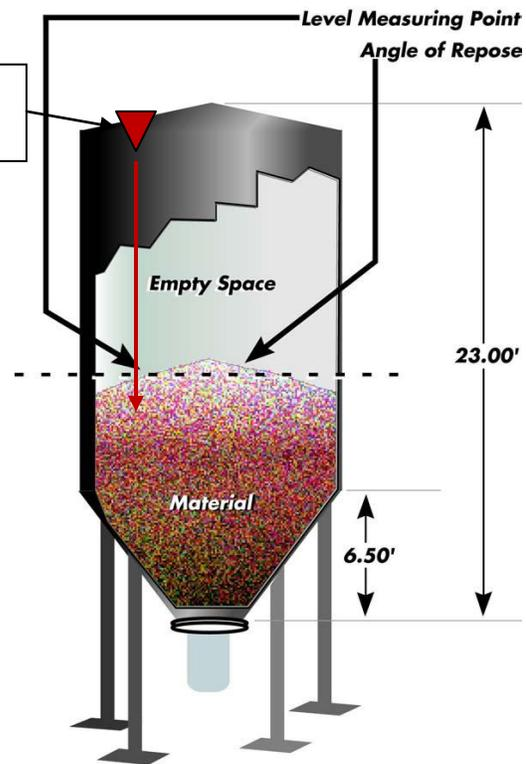
Figure 7: Sensor Location and Angle of Repose
