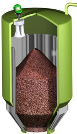
the location, if not the choice, of the continuous level sensor. For example, pneumatic filling of a powder introduces far greater dust into the vessel atmosphere than does gravity feeding the vessel. Heavier dust can impact the performance of **most** through-air level sensor technologies such as ultrasonic, laser and radar.
