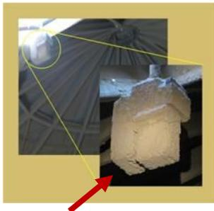
Figure 6: Laser Sensor Shown Inside Grain Bin, Covered with Grain Dust Even Though not in Material Flow Path or in Contact with Material Surface
