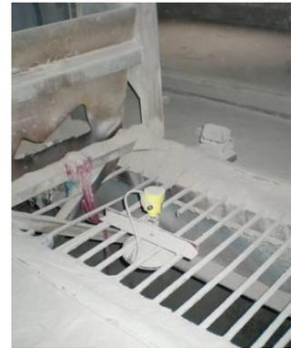
Figure 12: Open-air radar continuous level sensor measuring sintered powder
