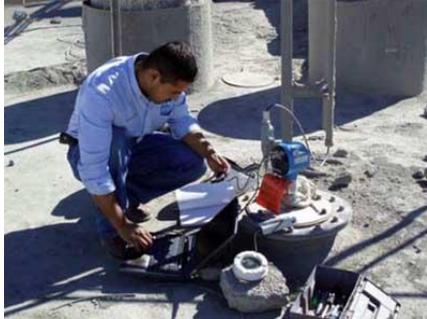
Figure 11: Technician Performs Start-Up Adjustments on GWR Device Measuring Flyash
