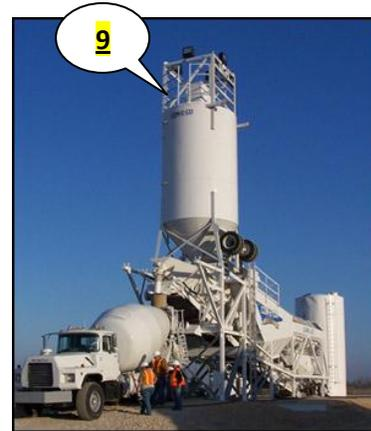
Figure 3: Portable concrete plant
