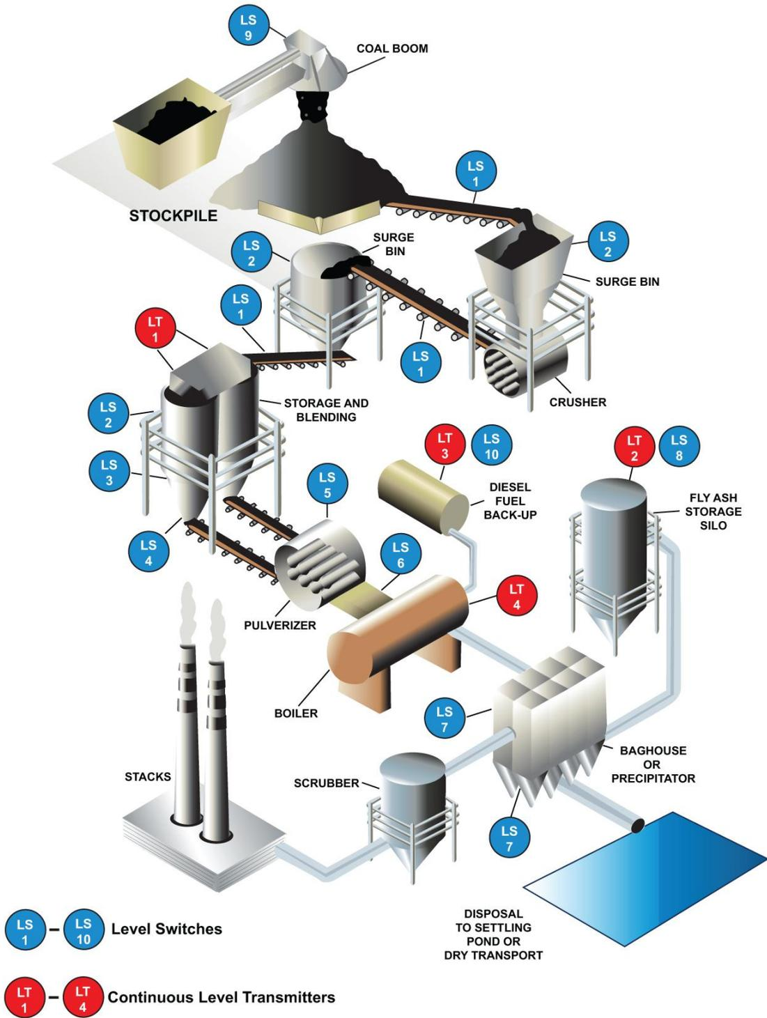
Figure 2: Level Sensing Process Diagram for Coal-Fired Power Plant
