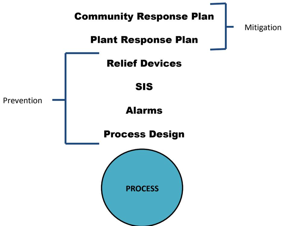
The specific layers of protection required will emanate from the Hazards Analysis. Such an analysis will include from an engineering study that reviews the process, electrical, mechanical, safety, instrumentation and management aspects of the process for those processes with severe risks. The Hazards Analysis will determine if an SIS is required. The purpose of the SIS, a.k.a. safety shutdown or safety interlock, is always to take the process to what is considered a minimal “safe state”.
