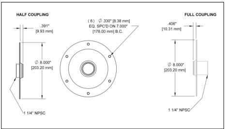
Full Coupling Mounting Plates are used for top mounting applications where an extension guard is used and is threaded into the underside of the Mounting Plate.
