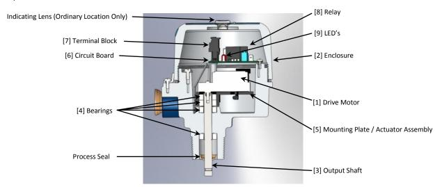
The unit's drive motor [1] is mounted within the enclosure on a spring-loaded mounting plate [5] with attached switch actuator. A circuit board [6] containing user terminal block connections [7], output relay [8] and high intensity LED indicators [9] is mounted above the drive motor assembly.
